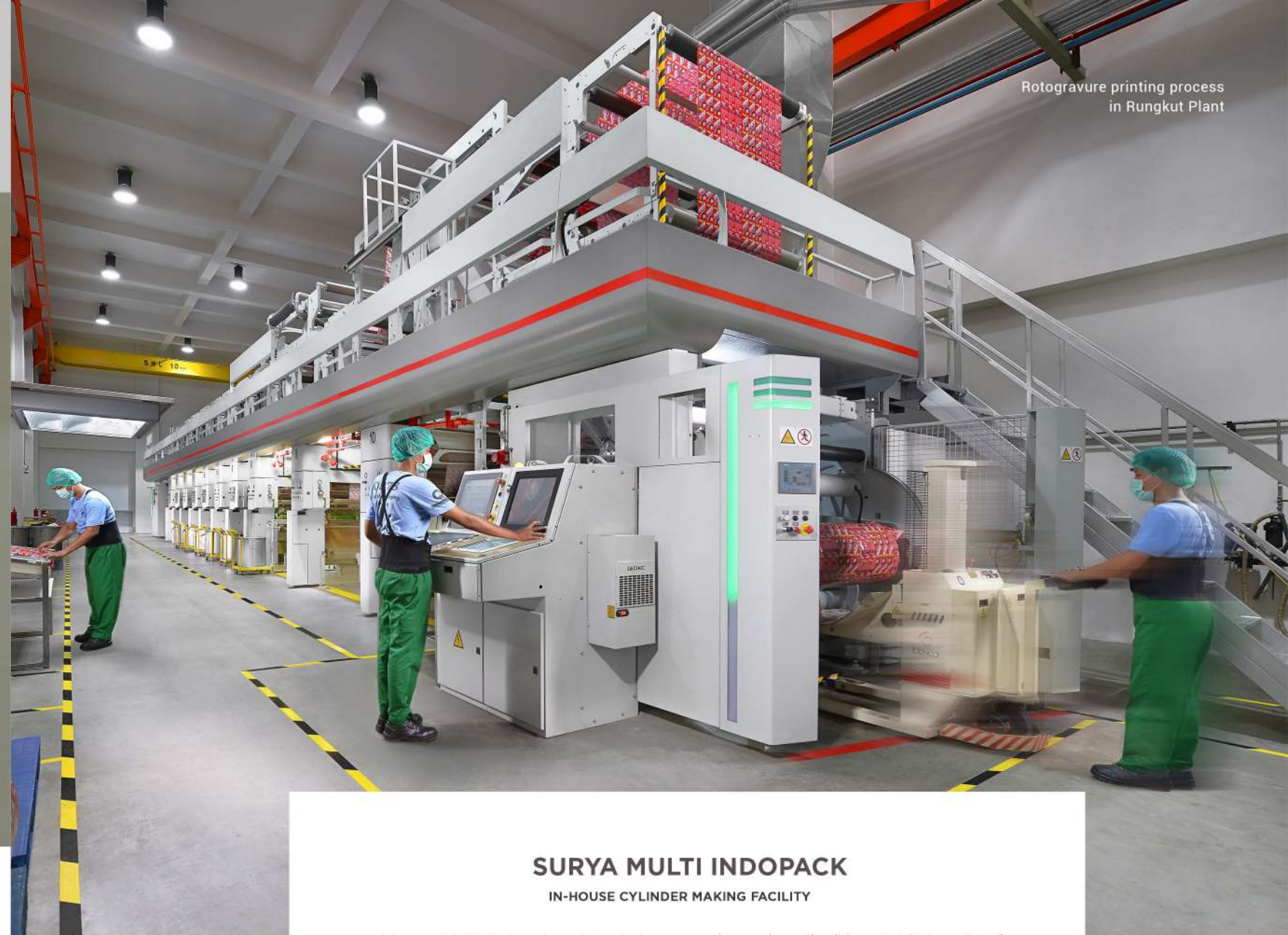
Ongoing register setting process at Rotogravure printing machine
