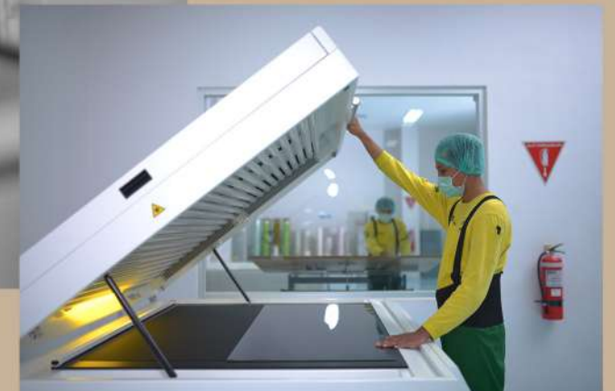
Plate making process for flexography print
