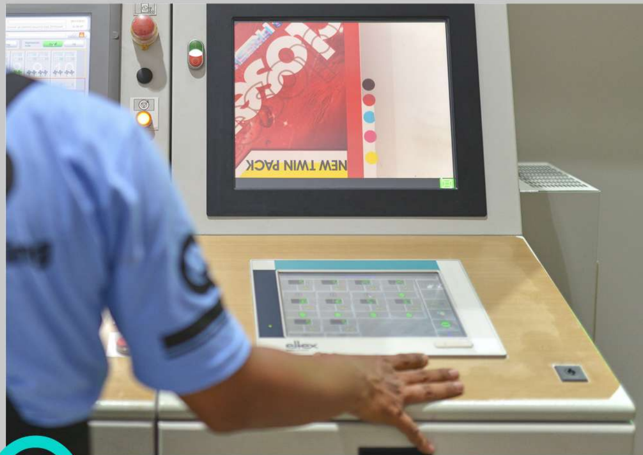
Ongoing register setting process at Rotogravure printing machine
